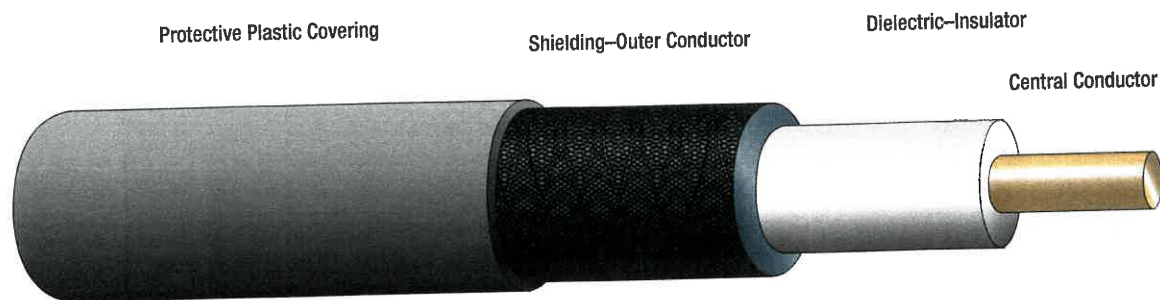
Figure 10-1. Coaxial cable typically used for data rates of 2Mbps to 50Mbps.
