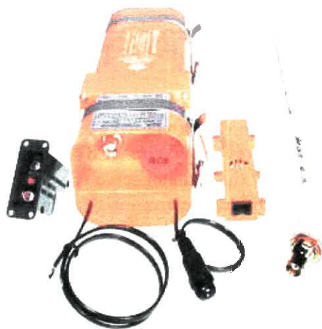
Figure 15-21. An ELT and its components including a cockpit mounted panel, the ELT, a permanent mount antenna, and a portable antenna.
