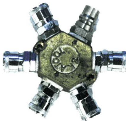
Figure 10-14. A six-port star coupler.
