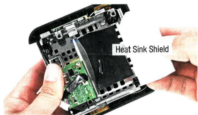
Figure 14-5. Heat-sink shield acts as a faraday cage to block electromagnetic emissions.
