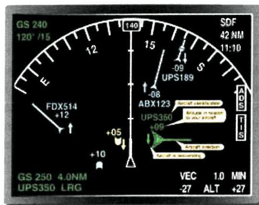
Figure 15-15. A cockpit display of ADS-B generated targets (left). ADS-B airborne receiver with antenna (right).
