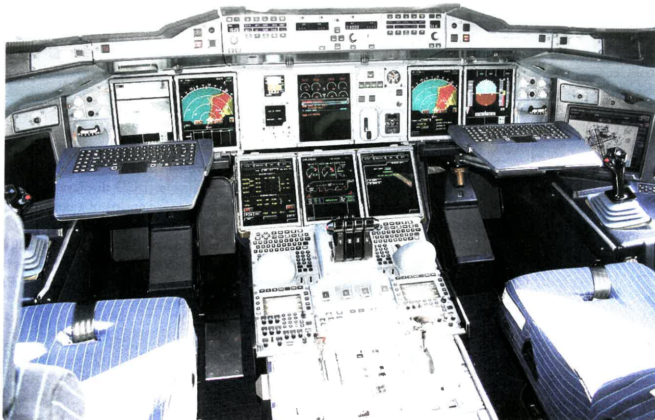
Figure 1-2. Airbus A380 EIS with 8 large LCD displays.
